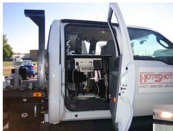
New HotShot 4WD Inspection vehicle fitted with Mattrack treads
